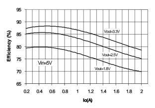
Figure 10. Efficiency vs. Output Current
