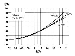
Figure 8. Junction Temperature vs Output Current
